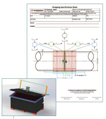
With DraftSight Professional software, Superheat not only can read in DWG files of customer products requiring heat treatment but can also manipulate drawing layers on heat-treatment designs to remove its sensitive IP from drawings or include it if clients choose to purchase drawings containing all lauers as part of their heat-treatment solution.
