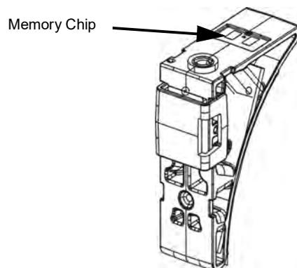
When a canister is installed, its memory chip is read and the canister's information is reported to the printer. The canister's material type and volume are displayed on the User Interface within the Dashboard (see ["Dashboard" on page 52](#) for more information) as well as the Tips page (see ["Working with the Tips Page" on page 72](#)). If a non-compatible canister is installed, an error will be displayed on the User Interface.
