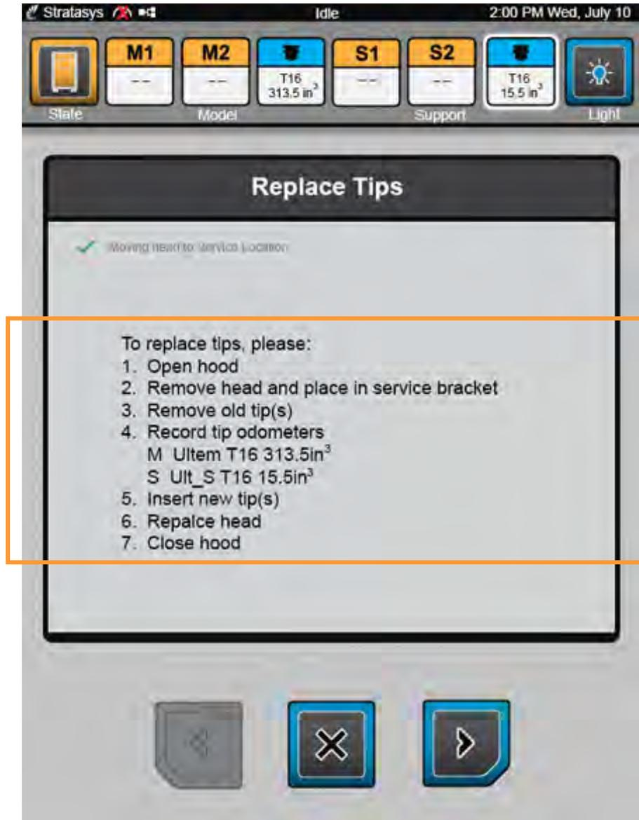
12. A default odometer value of 0.0 (in<sup>3</sup>) is automatically populated for the newly installed model and support tip; update tip odometer information as needed.
