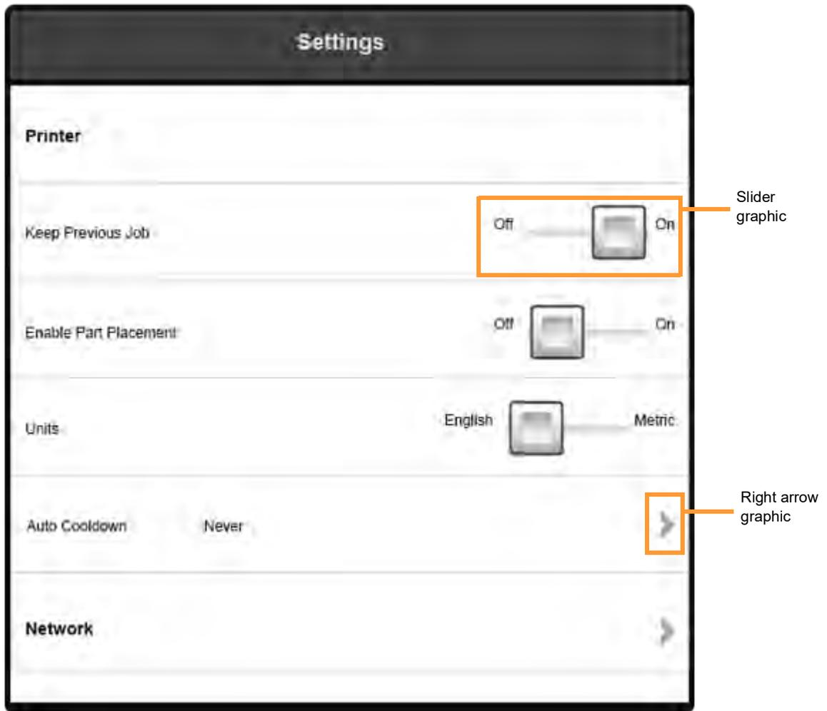
Rows containing a slider graphic (see Figure 4-39) allow you to configure a particular setting, typically turning the setting Off and On, directly within the Settings page. Simply touch the slider on the screen and move it to the left or right to adjust its setting.
