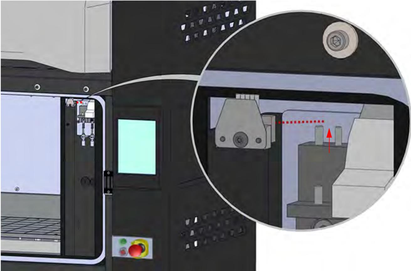
9. Clean and inspect the surface around the locating pins. Make sure that the purge ledges and flicker/brush assemblies can sit flush on the surface.
