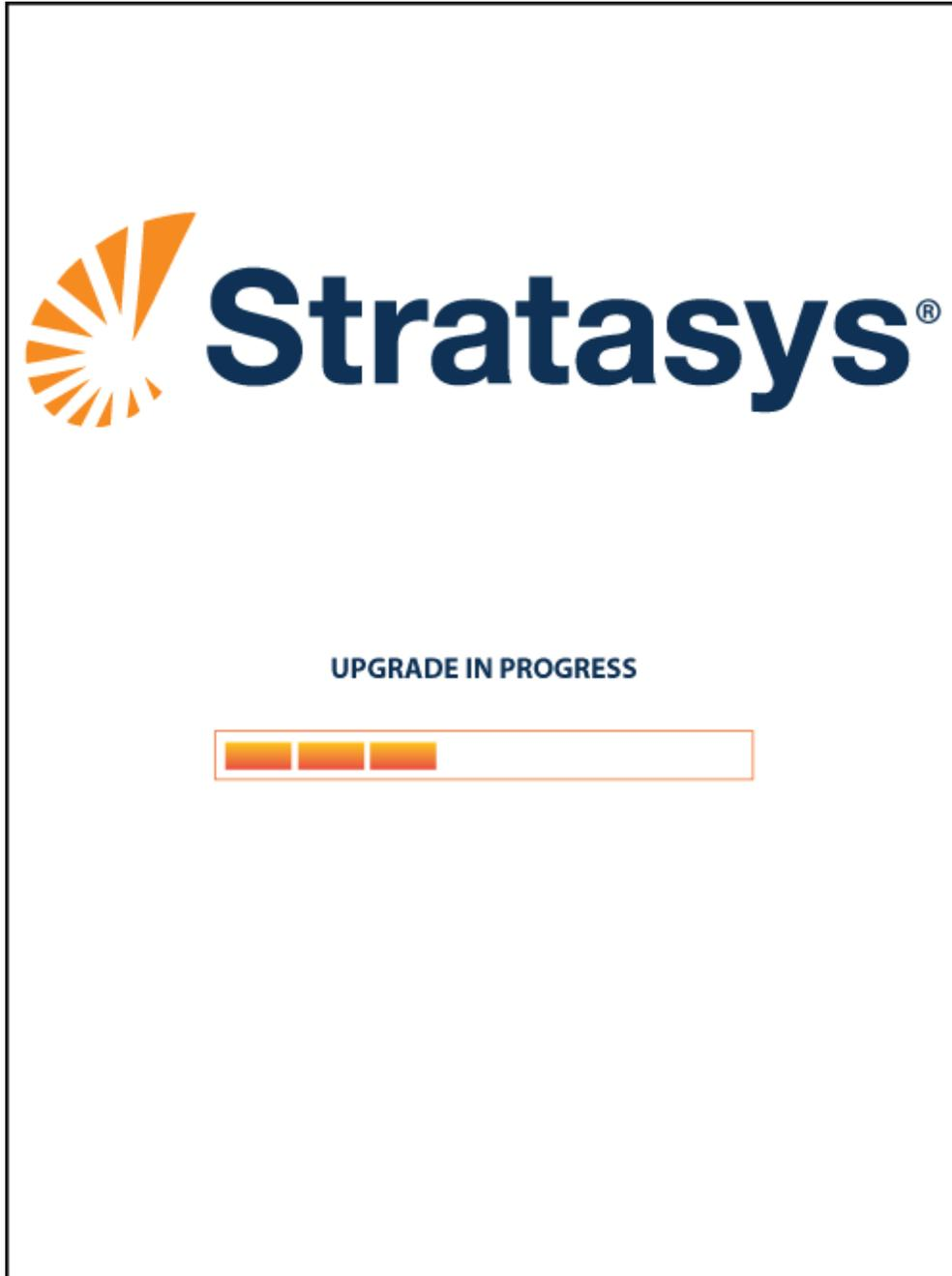
14. Once The printer reboots it will conduct its regular startup process and automatically perform an XY Home Calibration (see [“Powering ON the Printer”](#) on page 122 for details).
