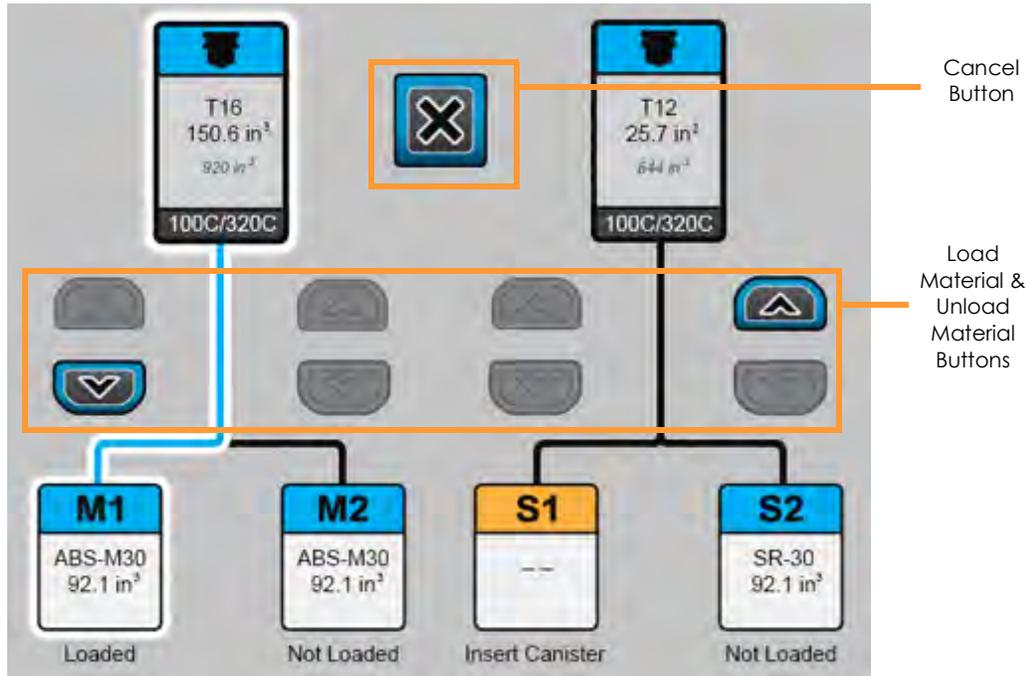
The Unload Material button (unselected state) will be selectable for all canisters with a "Loaded" status. The "Loaded" status is displayed for canisters whose filament is loaded to the corresponding liquefier tip in the head. Pressing this button will instruct the printer to begin the process of unloading material (see ["Unloading Material from the Liquefier Tips" on page 129](#) for details).
