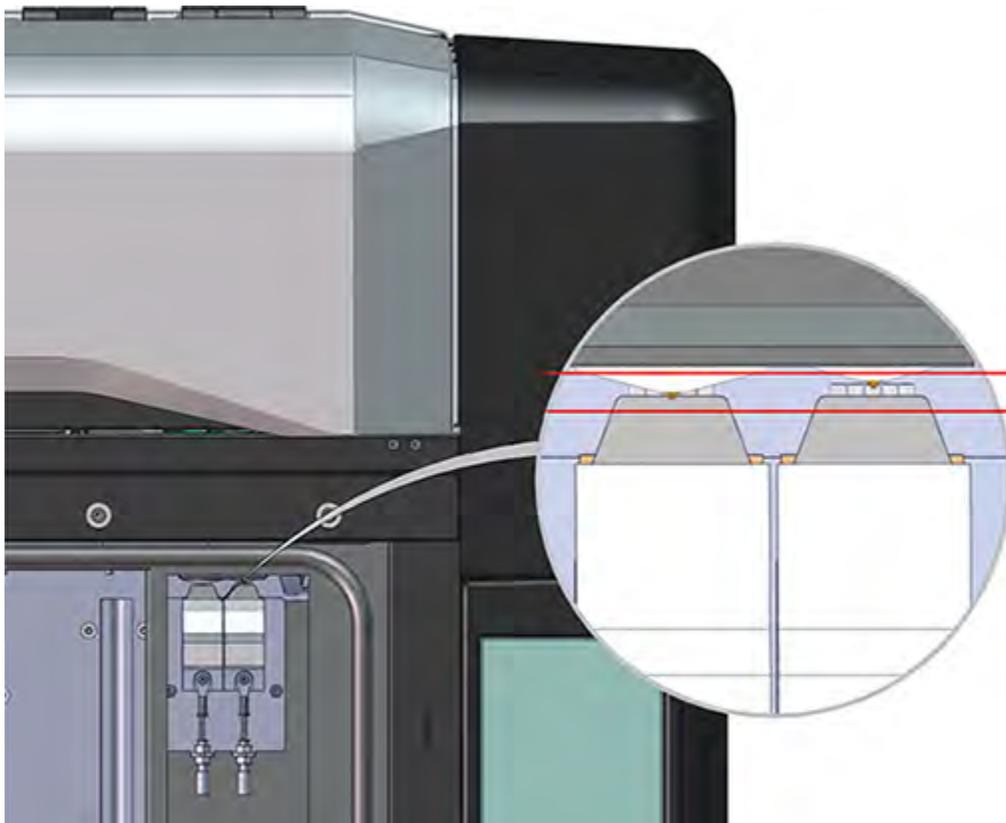
7. If additional adjustments are needed readjust height using the Tip Wipe Height Adjustment Wheels. When finished, close the canister bay doors.
