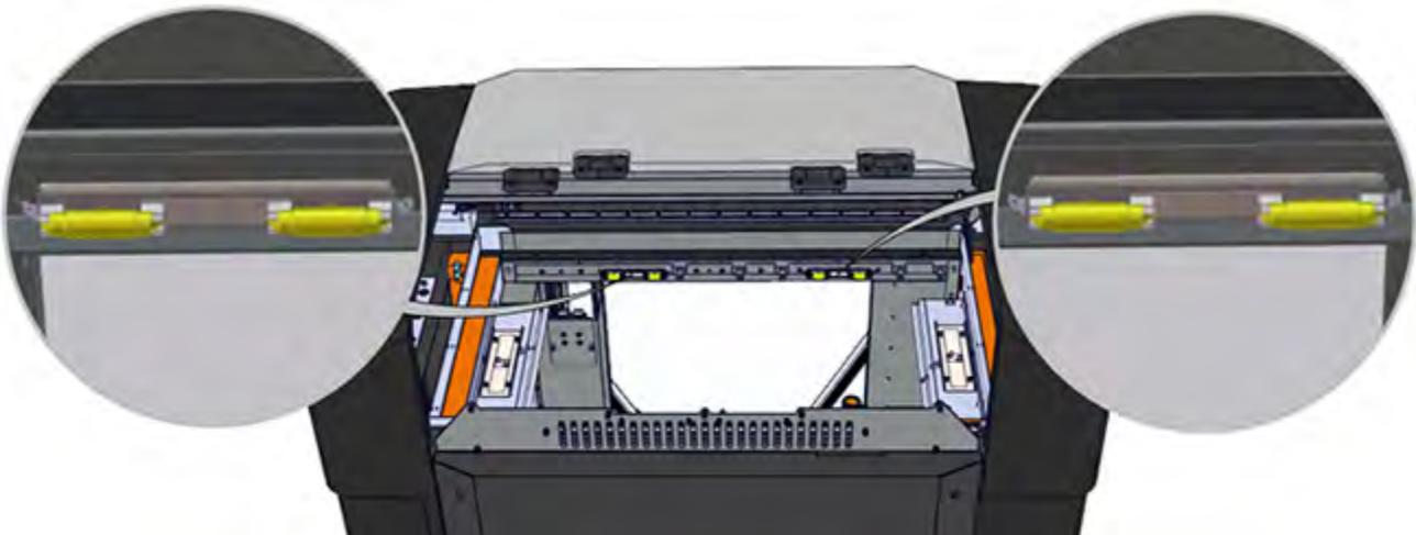
4. Install a replacement bulb by gently pressing it into place within the securing clamps.
