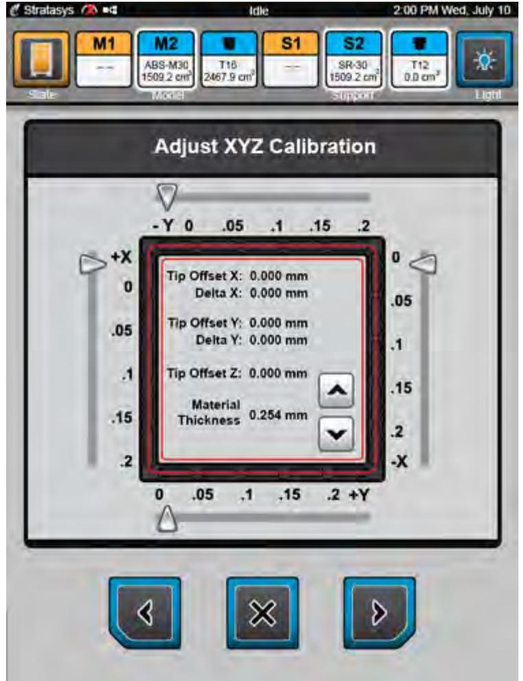
19. Determine the XY Offset Adjustment needed for your printer.
