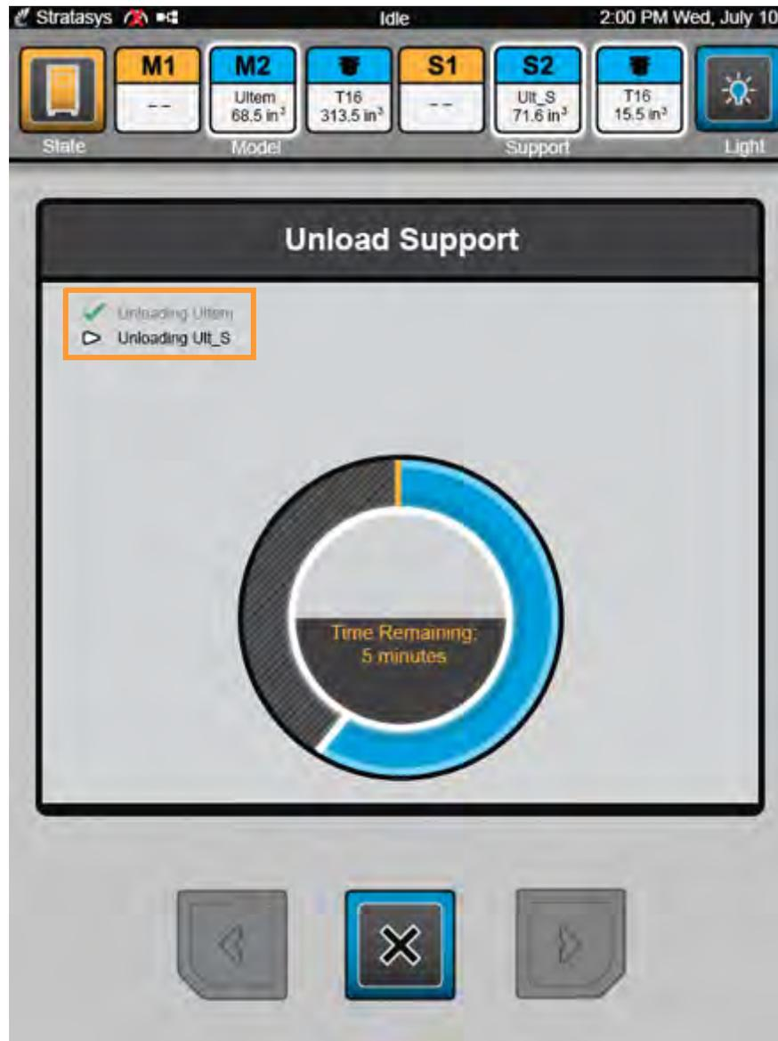
9. Once the material unload process is complete, you will be prompted to remove unloaded canisters (as appropriate). Remove unloaded canisters (see [“Removing Canisters”](#) on page 131) and then press the **Next** button to proceed with the wizard.
