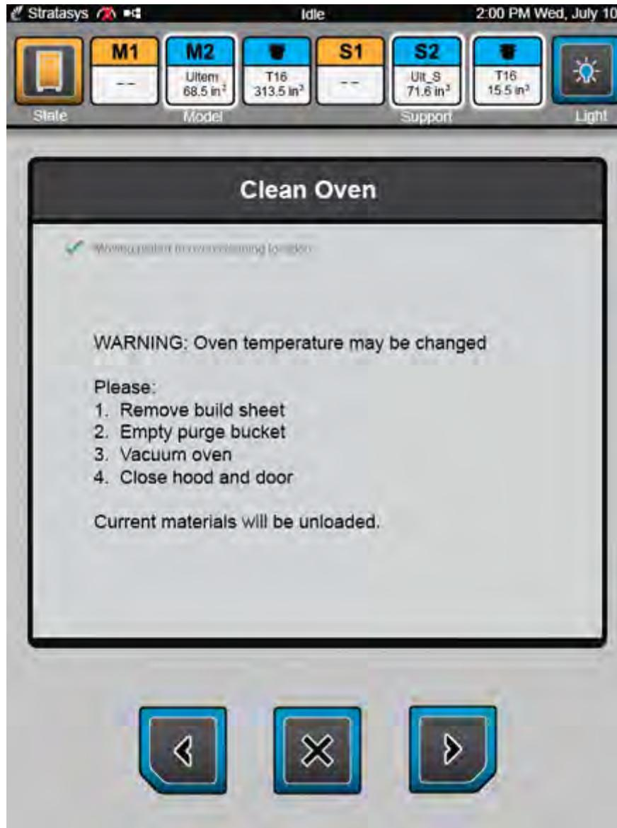
8. The model and support material currently loaded in the printer (Ultem and Ult\_S in this case) will start to unload (model material will unload first followed by support material). A two-part radial progress graphic displays the amount of time remaining until this process is complete (12 minutes in this case). Material unload percentage of completion is represented by radially filling in the outer progress ring of this graphic, in a clockwise direction.
