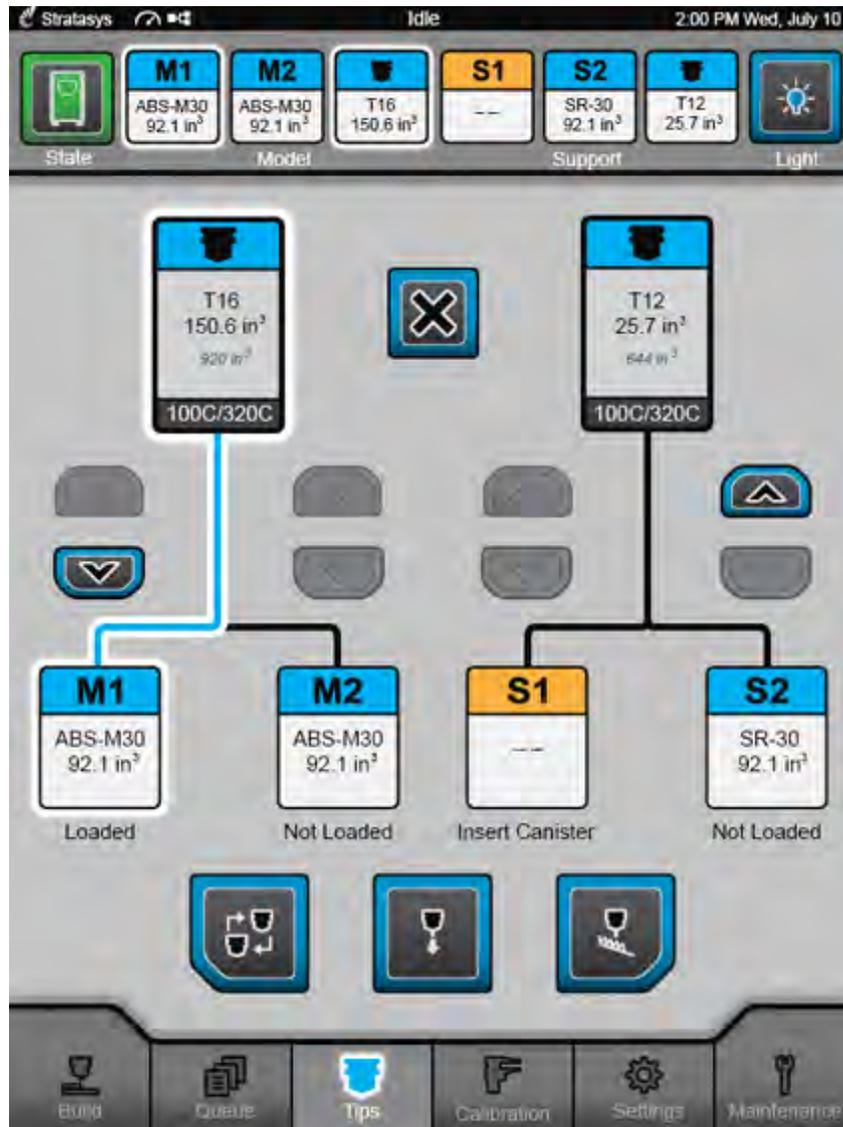
3. Observe the status information displayed below each of the model and support canister option icons. A "Loaded" status indicates currently loaded material.
