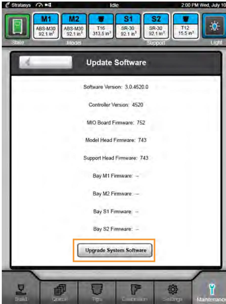
4. The following is displayed on the touchscreen while the printer is in Software Upgrade Mode. A radial progress graphic is displayed within the lower portion of the page, indicating that the printer is in Software Upgrade Mode and waiting to receive the software upgrade. The text displayed within this section of the page will update as upgrade progress is made.
