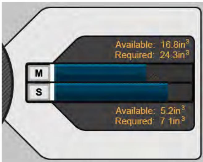
When the printer is building an additional progress bar is displayed for both the model and support fields. This light blue bar indicates build progress and reflects the amount of material used so far during the build.
