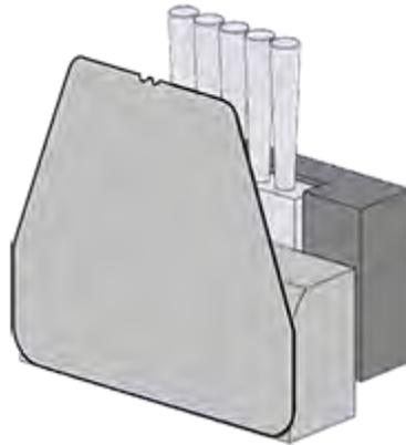
12. Inspect the brush portion of the flicker/brush assemblies. Brush bristles must not show evidence of wear (i.e. no notches in bristle pattern) and should not contain significant bristle clumping. Frayed bristles are acceptable as long as the top edge is even across all of the bristles.
