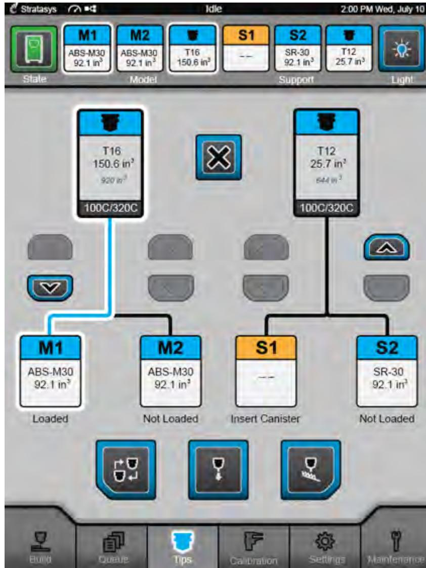
3. Observe the status information displayed below each of the model and support canister icons. The "Insert Canister" status indicates that a canister is not present in the material's corresponding canister bay.
