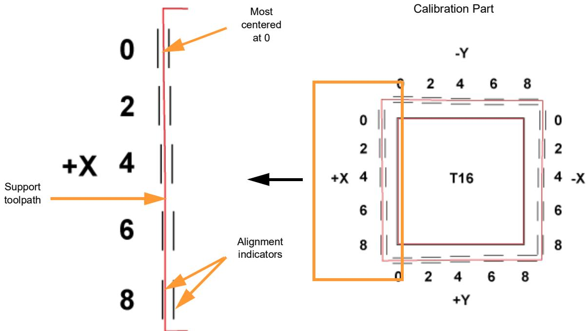
Figure 5-10: Calibration Part - Adjustment Needed (English units)
