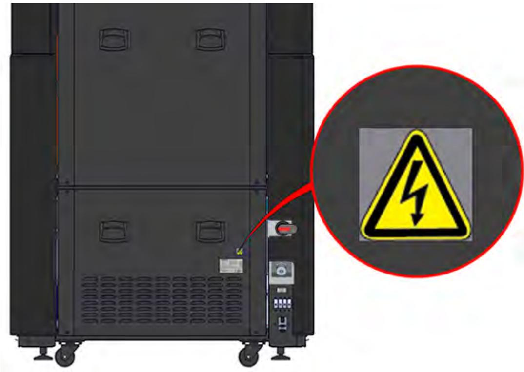
Figure 1-6: AC disconnect panel label locations
