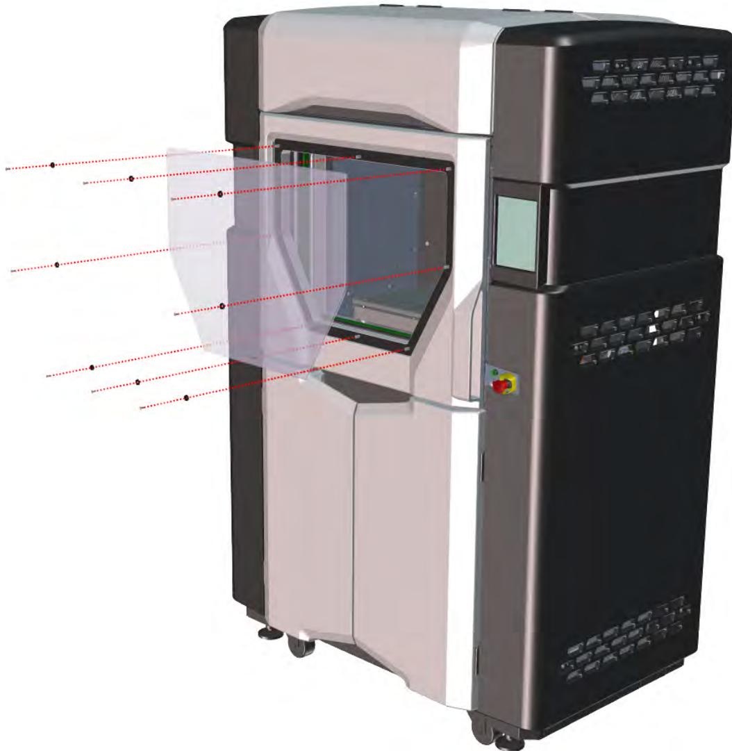
5. Gently clean the exterior surface of the tempered glass pane using a slightly soapy warm water solution, and a microfiber cloth (supplied in the Welcome Kit).
