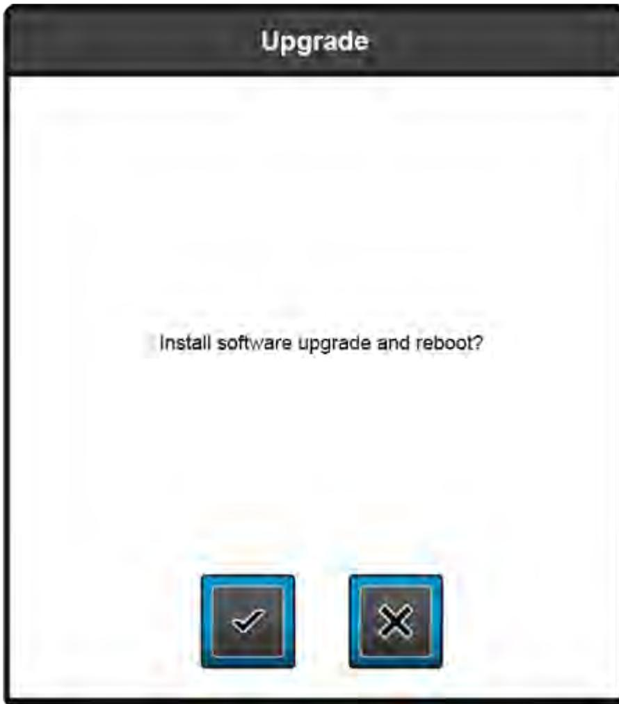
11. Controller Software will begin to boot on the printer. The following will be displayed on the touchscreen while the software update is booting on the printer.
