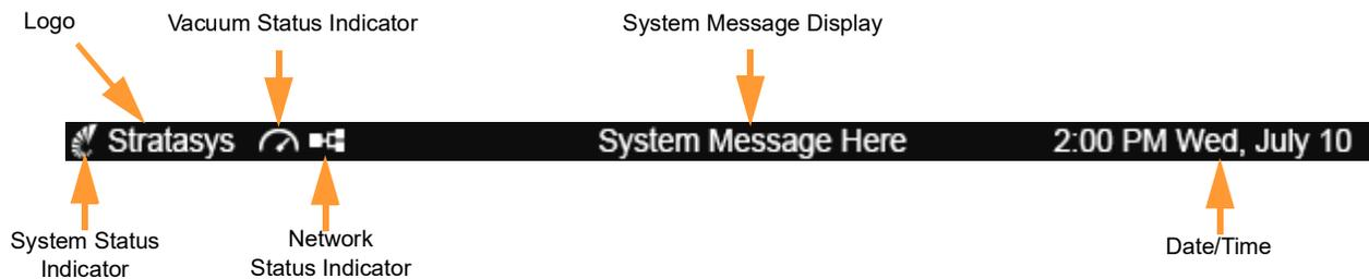
The System Status Indicator (nautilus shell icon) acts as the printer's "heartbeat"; when the printer is functioning correctly, the indicator will slowly flash on and off.
