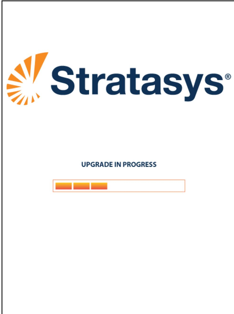
12. Once The printer reboots it will conduct its regular startup process and automatically perform an XY Home Calibration (see [“Powering ON the Printer”](#) on page 122 for details).
