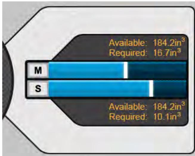
In [Figure 4-17](#), the light blue progress bars indicate the amount of model and support material used so far; however, there is not sufficient material in the printer to complete this build. The dark blue progress bars indicate the remaining amount of model and support available in the printer while the additional material required to complete the build is indicated in hashed-grey.
