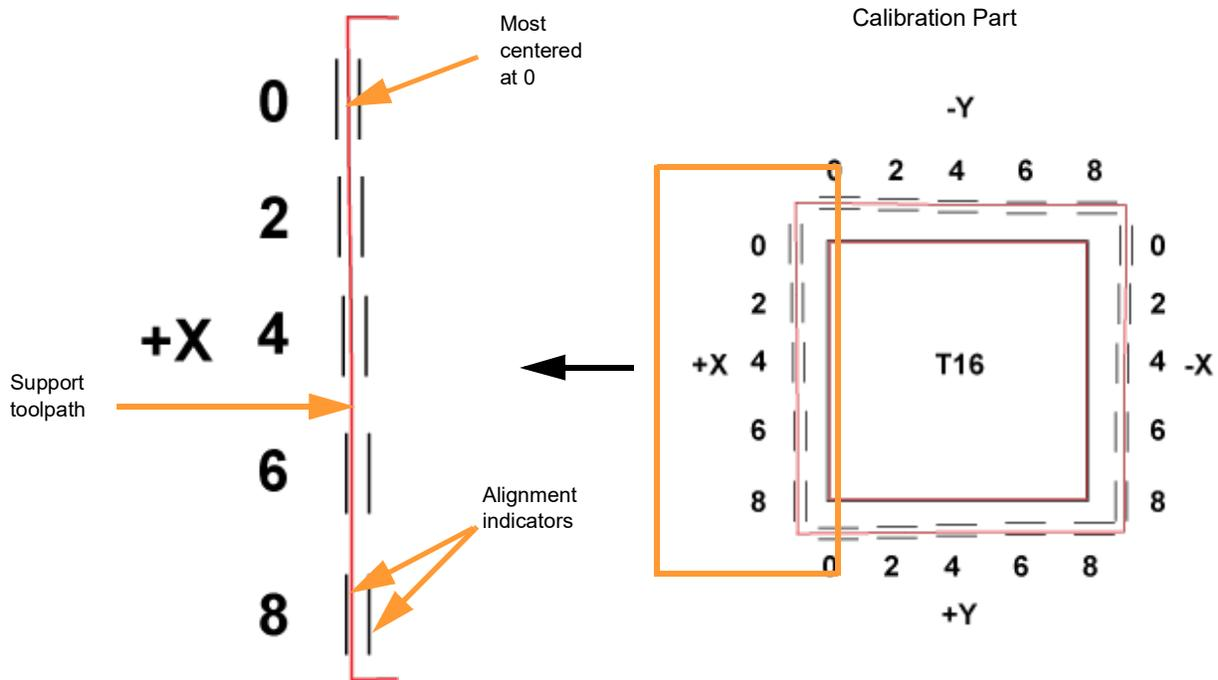
Figure 6-11: Calibration Part - Adjustment Needed (English units)
