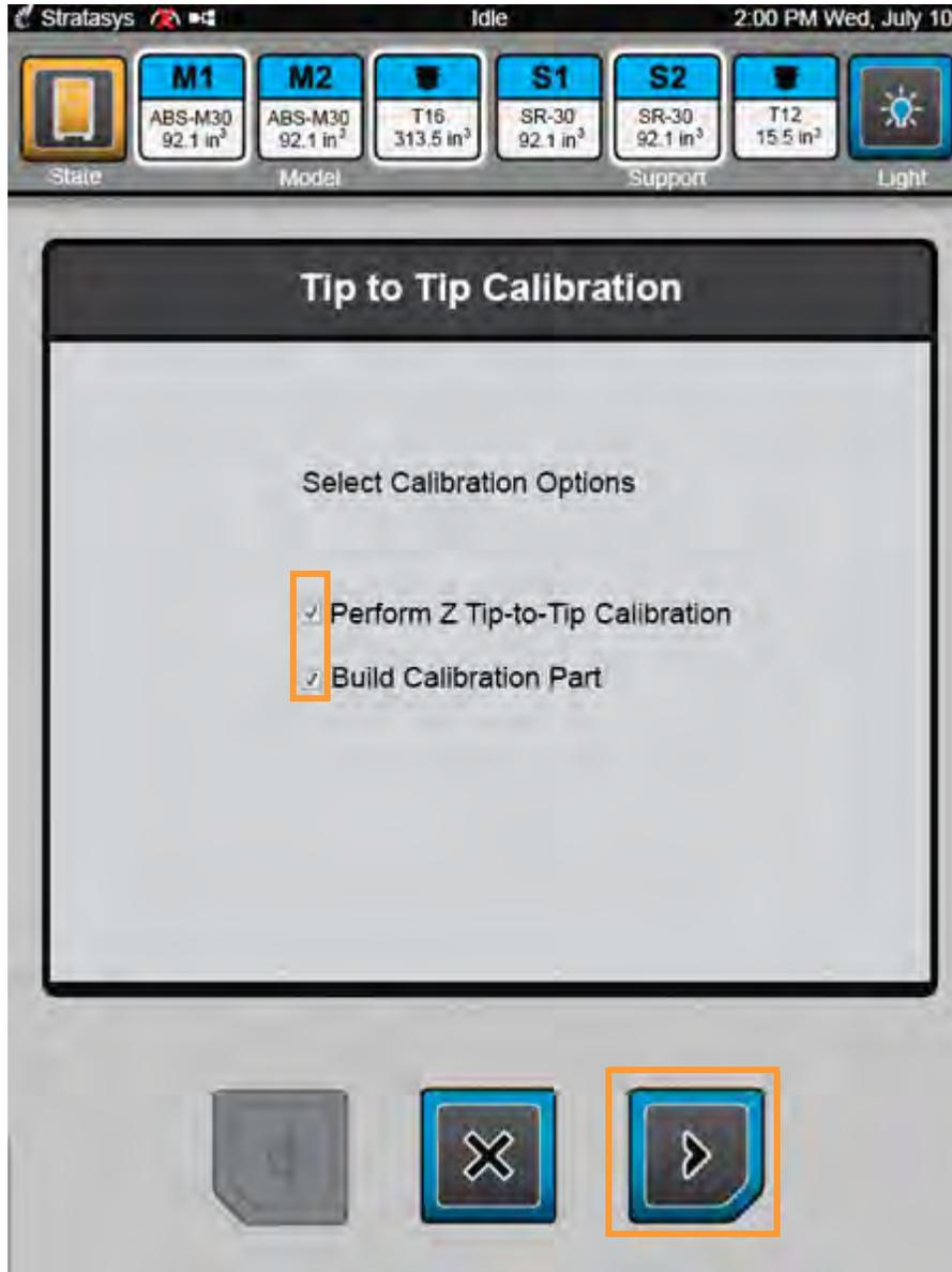
4. Perform the necessary steps to prepare for tip calibration and then press the Next button to proceed with the wizard.
