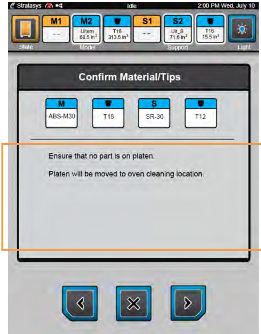
7. Once the platen moves to the oven cleaning location perform the steps displayed within the page. When finished, press the **Next** button to proceed with the wizard.
