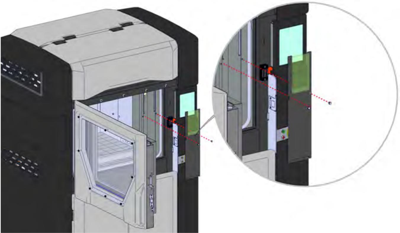
5. Remove the model side purge ledge by lifting it upward until it clears its locating pin.
