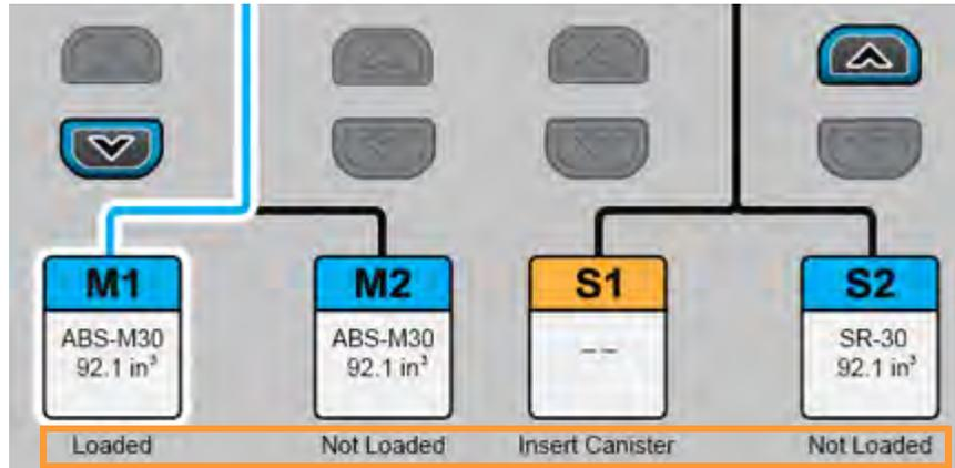
The various canister load statuses displayed are as follows:
