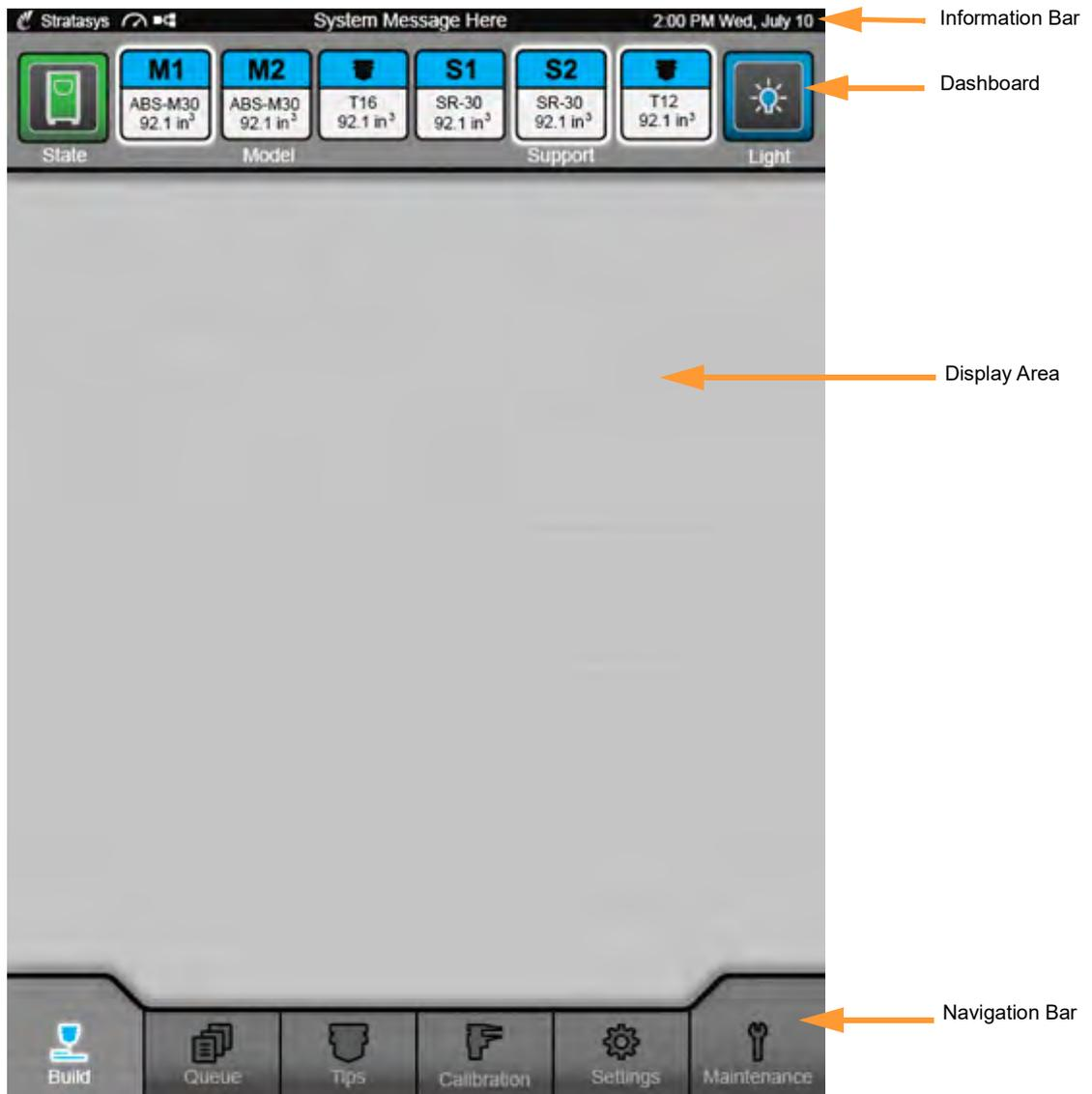
The touchscreen is designed to reduce glare; therefore, it is best to view the touchscreen when standing in front of the printer with the screen to your right. Viewing the touchscreen from any other angle may inhibit a clear view of the screen's display. The touchscreen is easy to use and allows you to:
