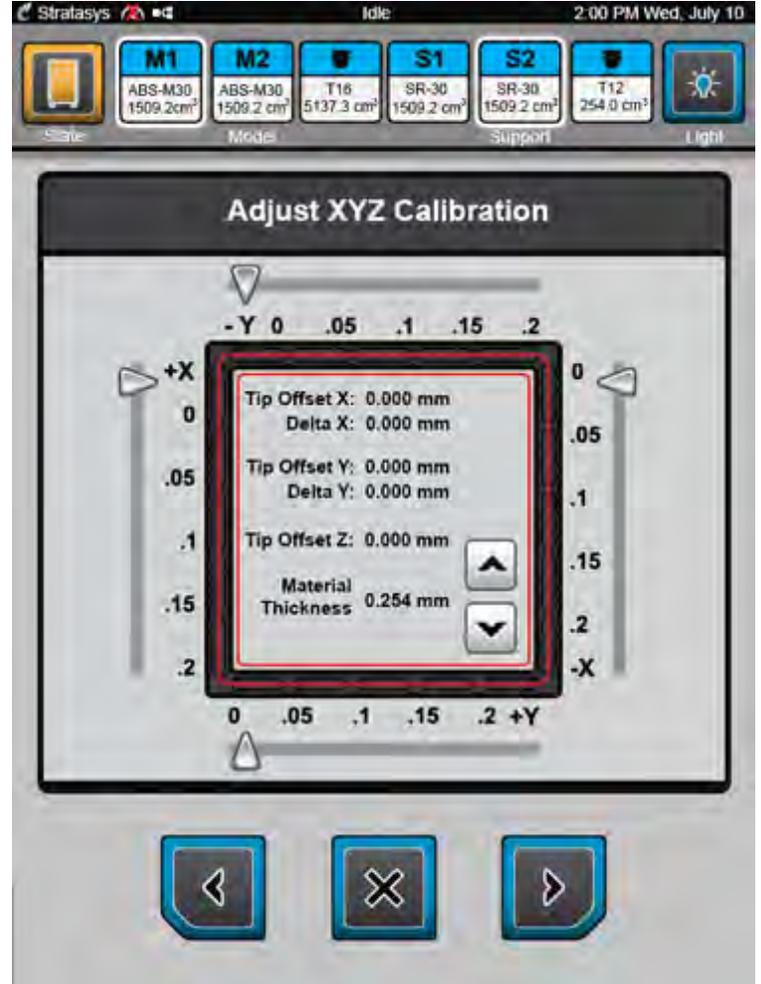
8. Determine the XY Offset Adjustment needed for your printer.
