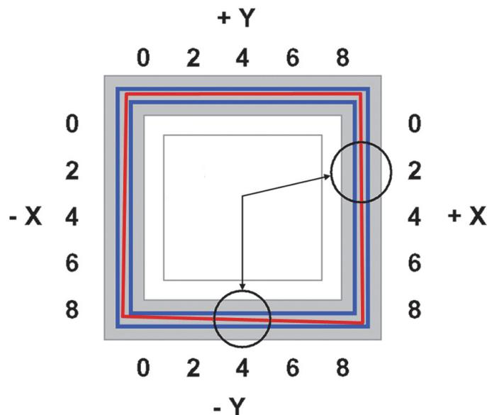
5. Select **Done** after you have input the X and Y offsets. The system will return to **Maintenance**. Run the XY calibration a second time to be sure the values changed the offset properly.
