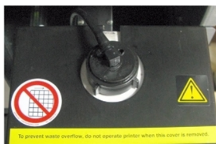
Figure 6-137 Cover installed on the waste container
