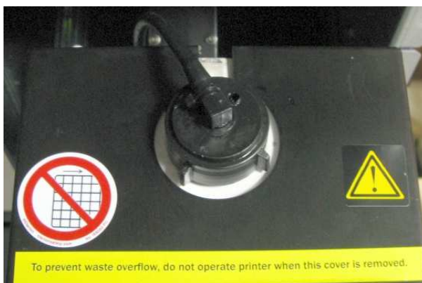
Figure 6-121 Cover installed on the waste container
