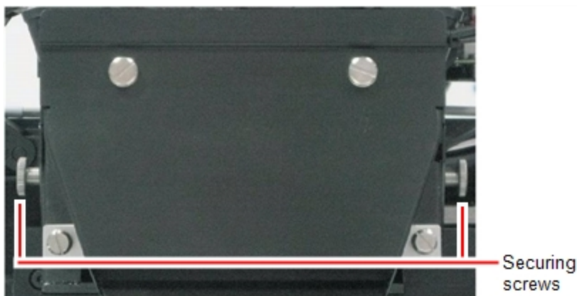
Figure 6-46 UV-lamp-assembly securing screws
