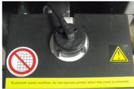
Figure 6-144 Cover installed over the waste container
