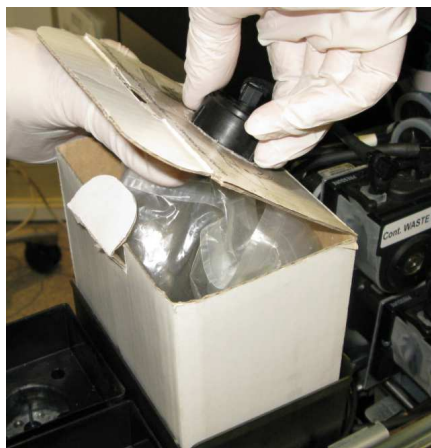
Figure 6-136 Waste container with waste tube attached
