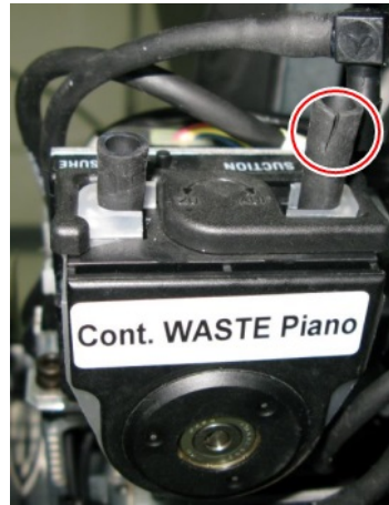
Figure 6-128 Tubes disconnected from the waste pump
