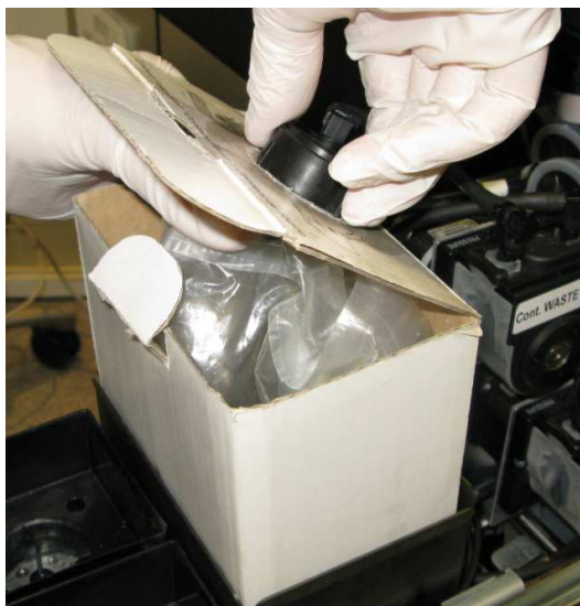
Figure 6-120 Attaching the waste drain tube
