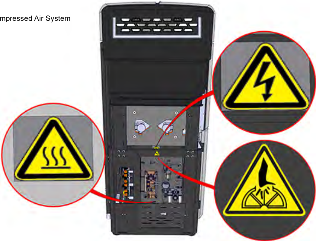
Figure 1-4: Air system safety label locations
