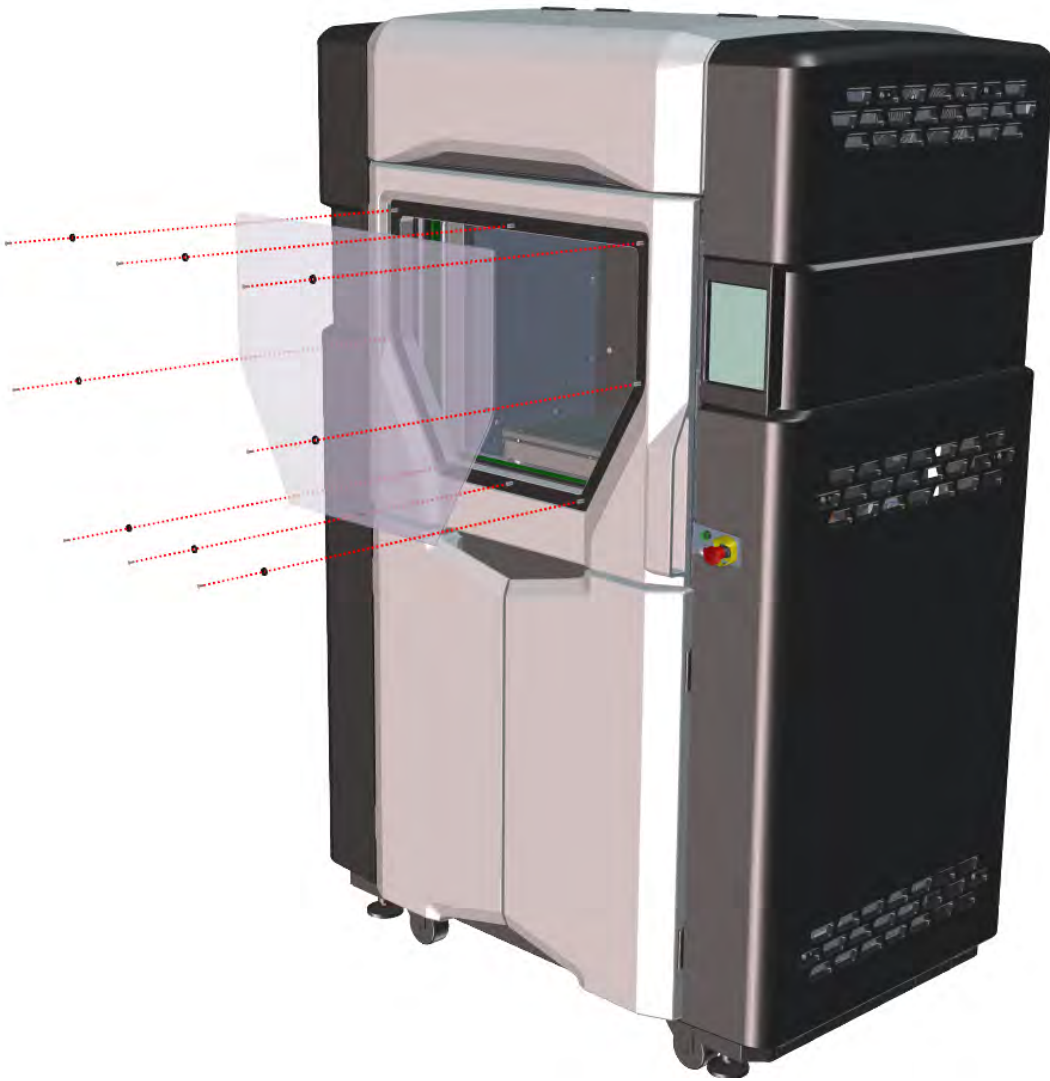
Figure 7-33: Removing Oven Window
