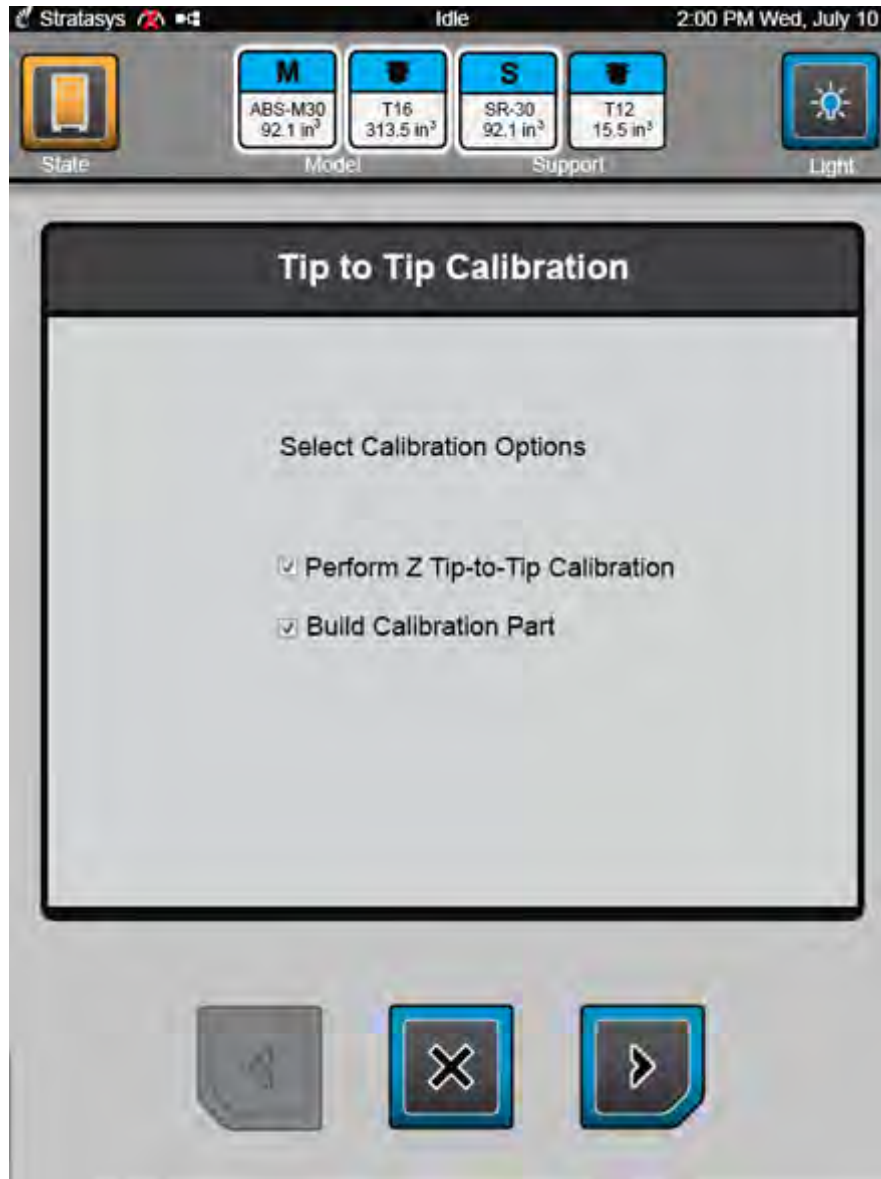
Figure 4-35: XYZ Tip Offset Calibration Page
