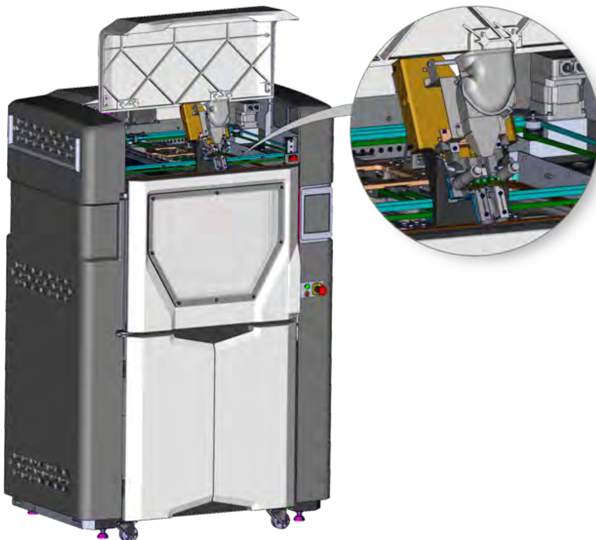
Figure 5-18: Head in Maintenance Bracket
