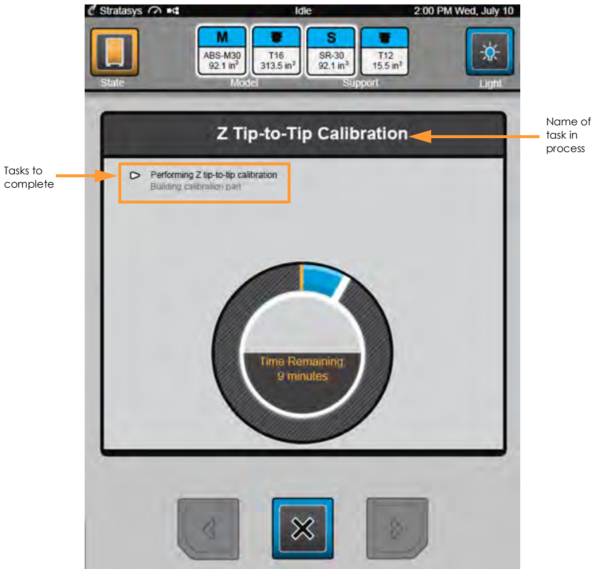
Figure 6-6: Z Tip-to-Tip Calibration Page
