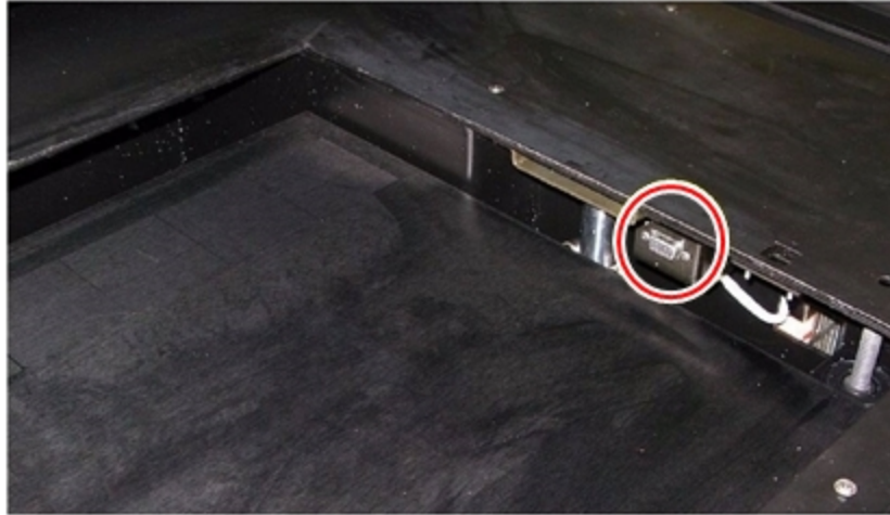
Figure 6-92 UV sensor connector
