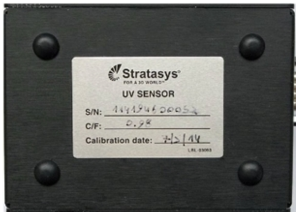
Figure 6-91 Label on the bottom of the UV sensor box
