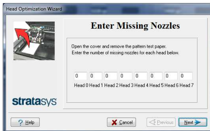
Figure 6-60 Enter Missing Nozzles screen
