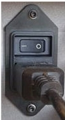
Figure 6-2 Main power switch and cable
